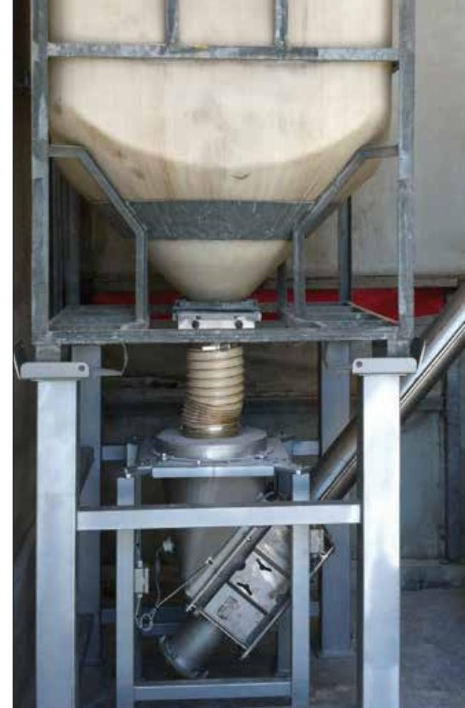
Special pick up from polyethylene tanks
