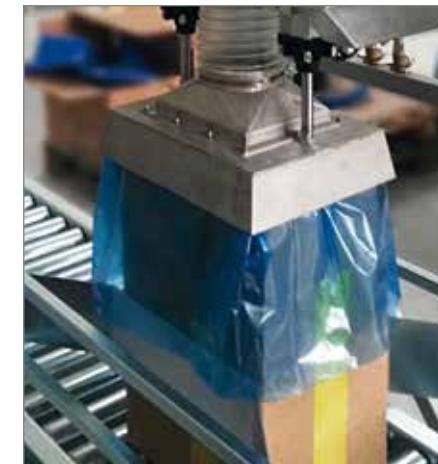
25 kg open mouth bag/box semi-automatic filling including: bulk bag unloading, sieving, metal detecting and dust extraction.
