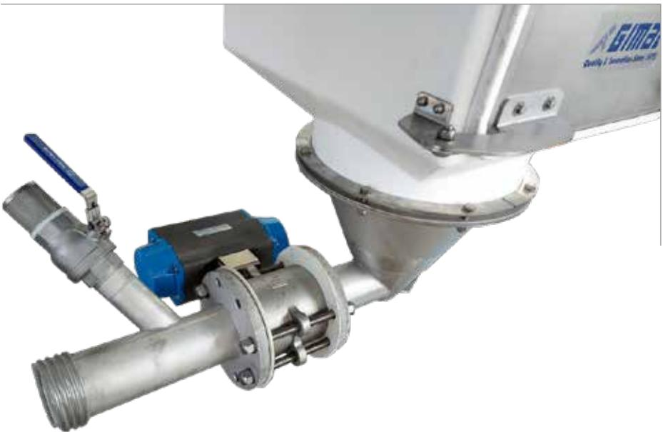
Pick up suction cone with 4" electropneumatic ball valve
