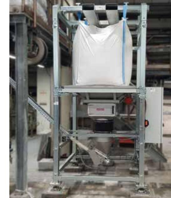
Bulk Bag Unloaders on load cells
