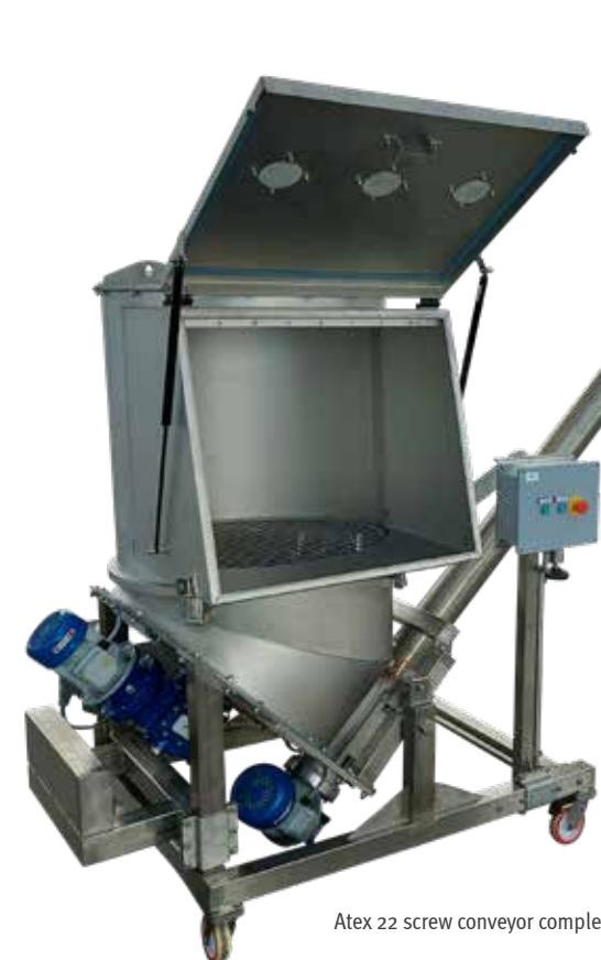
Atex 22 screw conveyor complete with bag emptying hopper
