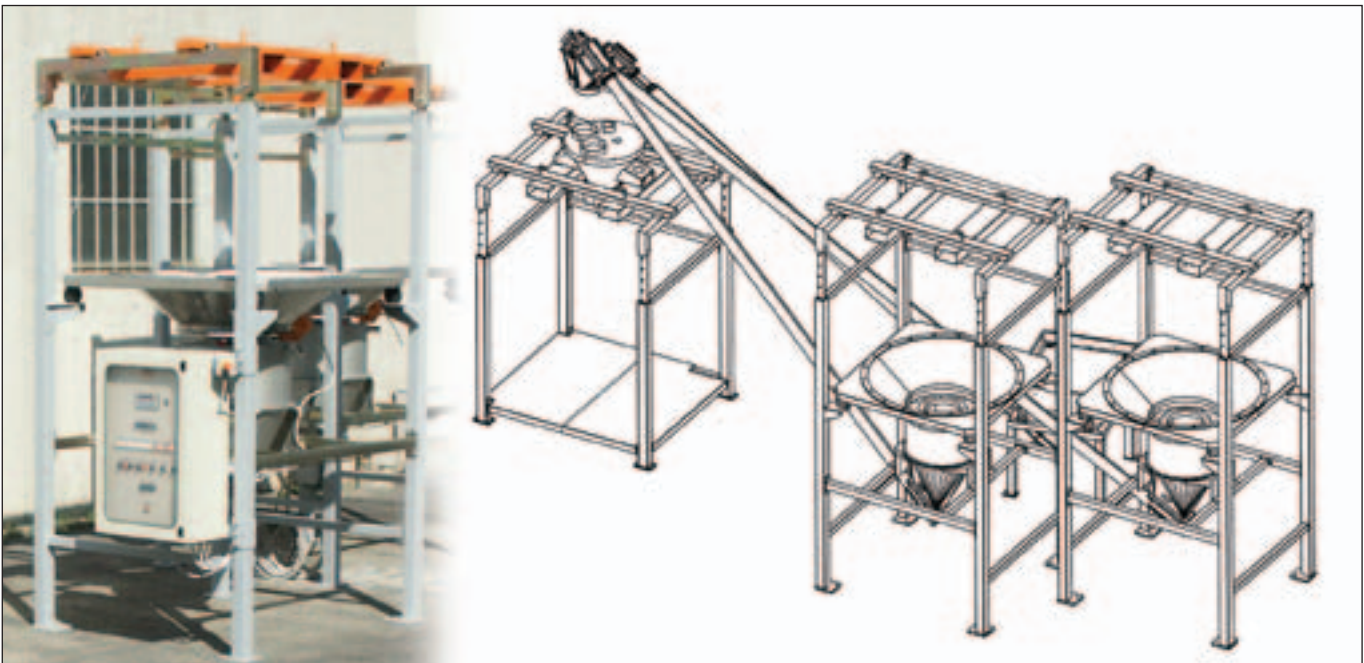
Plant for Bulk Bag - hopper with micro-components unloading and subsequent batching directly in the Bulk Bag filling station on loading cells
