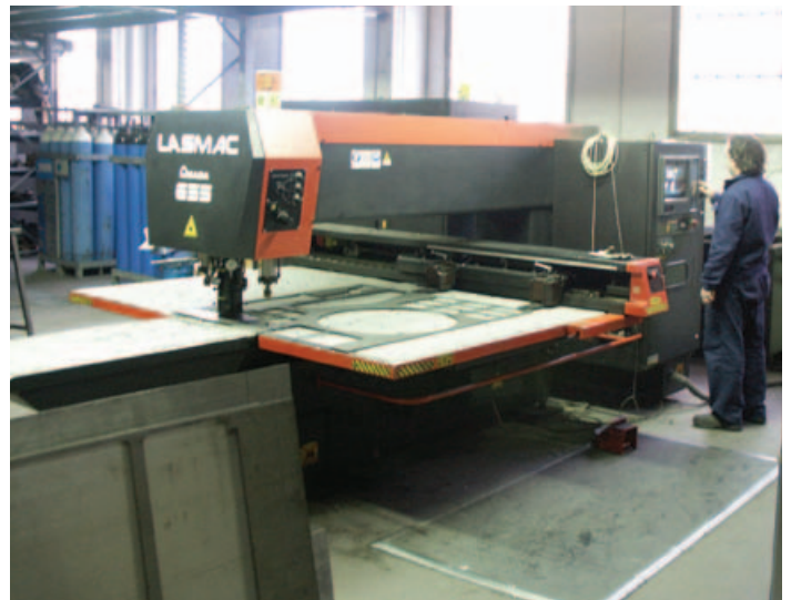
Processing sheets using laser cutting
