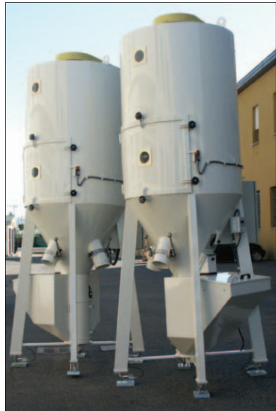
2000 lt Vertical Screw Mixers on load cells
