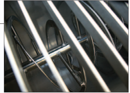
Agitator-Mixer interior detail
